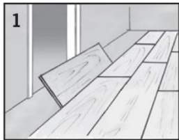
1 Some long edge joints cannot be installed using a 20° angle.
